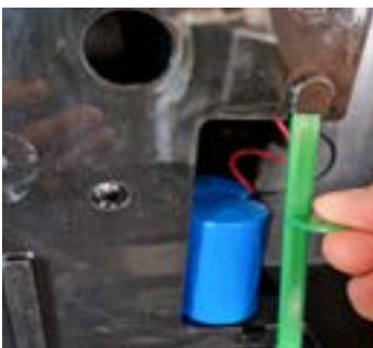
Remove the battery holder, pull out battery and replace.
