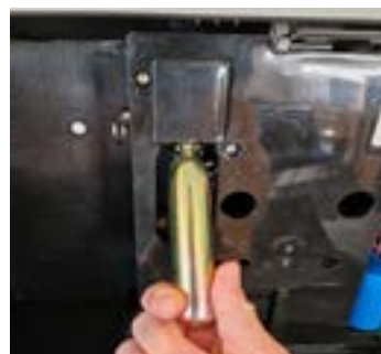
Unscrew co2 cartridge and replace (tighten new cartridge)
